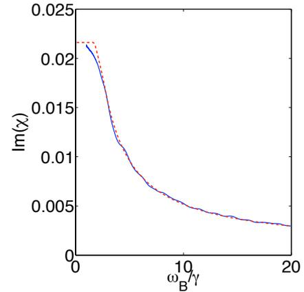
Figure 2:  $\text{Im}(\chi)$  calculated theoretically (red dashed line) and from a test particles simulation (blue solid line) when  $\gamma = 10^{-2} \omega_{pe}$  and  $\nu_\phi = 3\sqrt{T_e/m}$ .
