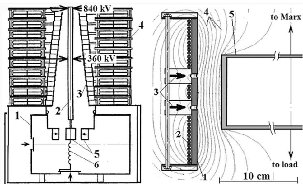
FIG.1. RS-20 generator, 1 – vacuum chamber, 2 – current drive, 3 – insulator, 4 – Marx, 5 – POS, 6 – load.
