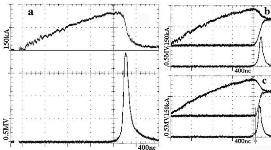
FIG. 5 signal waveforms, a – open circuit, b – current switching to the load  $L_H=0.32L_0$ , c – current switching to the load with separating switch.
