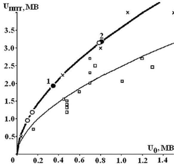
FIG. 6. Dependence of  $U_{POS}$  on  $U_{Max}$ . Top curve ( $\times, \circ, \bullet$ ) – for the POS in applied magnetic field, bottom curve ( $\square$ ) – for the experiments without magnetic field. Points « $\bullet$ » (1, 2) were obtained at RS-20, points « $\circ$ » were obtained in the previous experiments.
