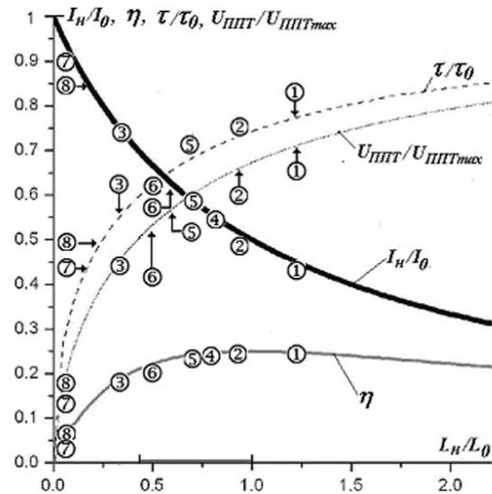
FIG. 7. Calculated and experimental values of the  $I_{load}/I_0$ ,  $\eta=L_{load}I_{load}^2/L_0I_0^2$ , current front  $\tau/\tau_0$ , POS voltage ratio  $U_{POS}/U_{POSmax}$  as functions of arbitrary load inductance  $L_{load}/L_0$ .
