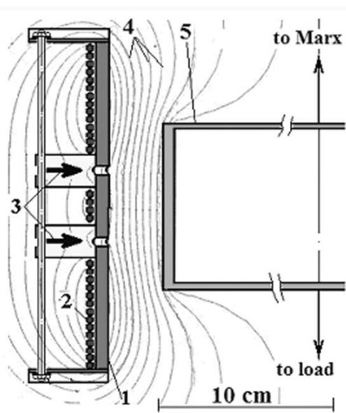
Fig. 2. POS scheme, 1–cathode, 4–solenoid, 5– plasma guns, 6 – magnetic field lines, 7 – anode
