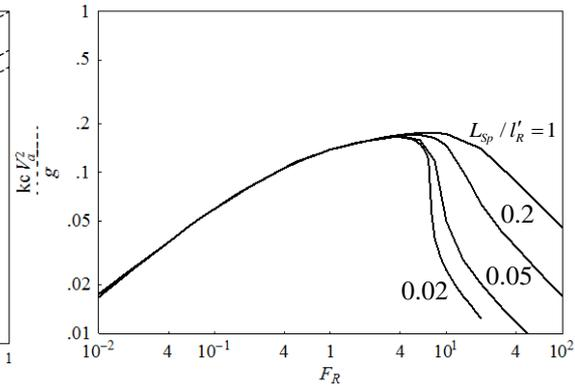
FIG.4. Normalized cutoff wave number versus Froude number for several values of  $L_{Sp} / l'_R$ .
