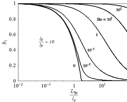
FIG.1. The function  $b_1$  versus  $L_{Sp}/l_p$  for several values of the Boltzmann number  $Bo$ .
