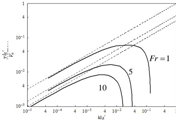
FIG.3. Normalized linear growth rate versus normalized wave number for several values of the Froude number and  $L_{Sp} / l'_R = 1$ . The dashed straight line correspond to the classical RT,  $\gamma = \sqrt{kg}$ .
