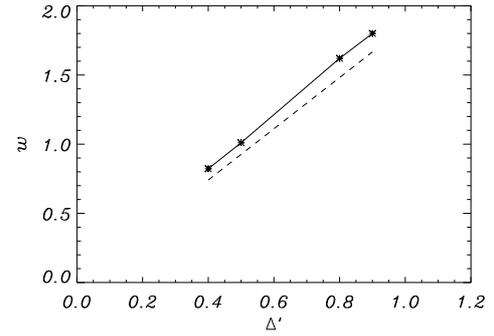
Figure 1: Island width as function of  $\Delta'$  for symmetric tearing modes with  $\alpha = 0$ . The numerical data are represented by the asterisks, while the analytical prediction is represented by the dashed line.
