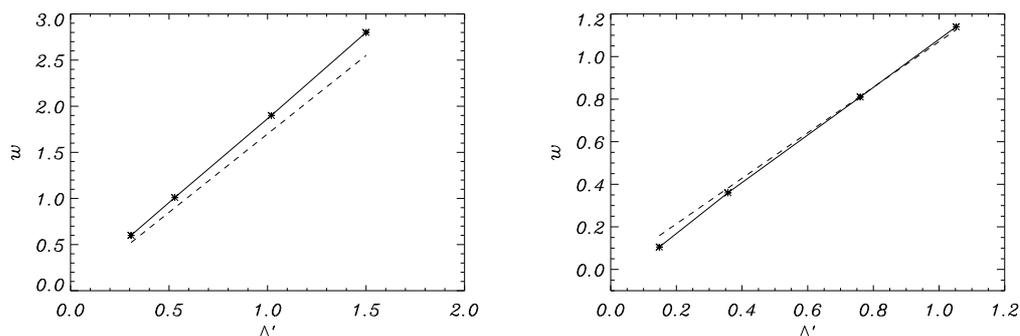
Figure 2: Island width as function of  $\Delta'$  for asymmetric tearing modes with  $\alpha = 0.2$  (left frame) and  $\alpha = 0.577$  (right frame). The numerical data are represented by the asterisks, while the analytical prediction is represented by the dashed line.
