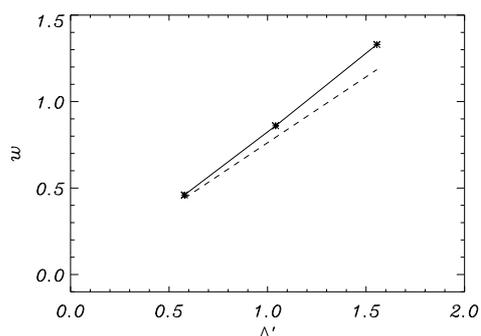
Figure 3: Island width as function of  $\Delta'$  for asymmetric tearing modes with  $\alpha = 0.8$ . The numerical data are represented by the asterisks, while the analytical prediction is represented by the dashed line.
