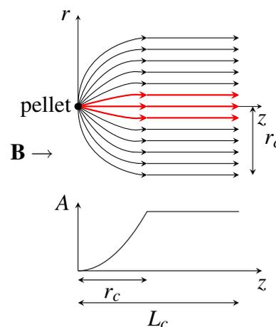
Figure 1: The initial spherical, then field aligned expansion of the pellet cloud, and the quasi 2D geometry.
