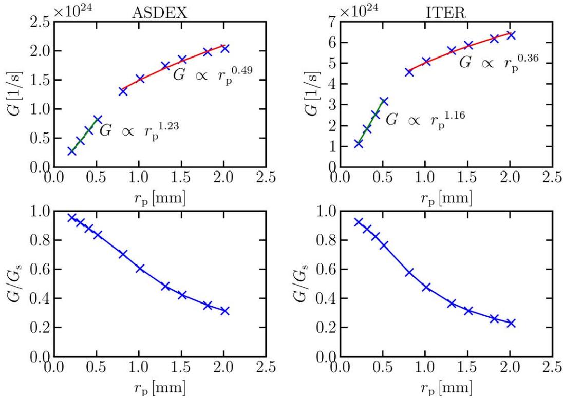
Figure 2: Ablation rates ( $G$ ) and ablation rates compared to the corresponding spherical symmetric expansion ( $G_s$ ) at different pellet sizes for the two model scenarios.
