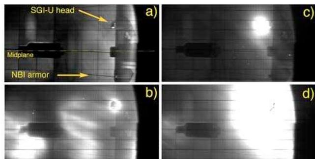
**Figure 1:** Fast camera images of jet-plasma interaction: (a) SGI-U head in the vacuum vessel at  $R = 1.57 \text{ m}$ , (b) Plasma interaction with SGI-U head during an MHD event, (c)  $D_\alpha$  emission from jet in the initial phase of high-pressure injection, (d)  $D_\alpha$  emission during high-pressure injection.
