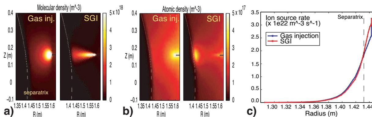
**Figure 5:** DEGAS 2 simulations of the conventional and supersonic gas injections in the H-mode plasmas: (a) molecular, (b) atomic densities, (c) flux surface averaged ionization rates. An artificial elongation 2:1 was given to panels (a) and (b) for clarity.
