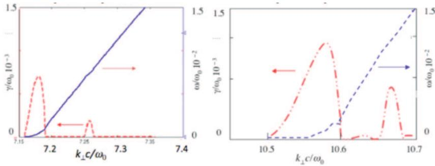
Fig. 2. Growth rate (in red) and frequency (in blue) of the quasimode driving PI relevant for the spectral broadening for the two different operating frequencies proposed for LHCD in ITER:  $f_0 = 5$  GHz (fig a), and  $f_0 = 3.7$  GHz. Operating parameters:  $n_e = 10^{18} \text{ m}^{-3}$ ,  $T_e = 25 \text{ eV}$   $n_{||0} = 1.8$  (pump wave),  $n_{||} = 3$  (ion-sound quasimode),  $B_T = 4 \text{ T}$ .
