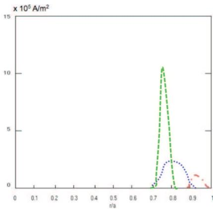
Fig. 3. LHCD deposition profile obtained in the Case 1 (see the text, dotted-dashed line), Case 2 (dotted), and no spectral broadening (dashed).
