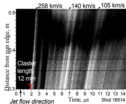
Fig.3: Propagation of the jet radiation recorded with a streak-camera
