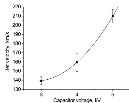
Fig.4: Dependence of the jet velocity on voltage at the capacitor
