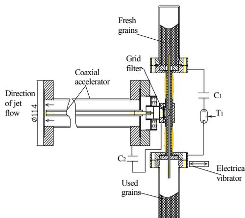
Fig.1: Two stage plasma gun, with explosive method of gas feeding a coaxial accelerator
