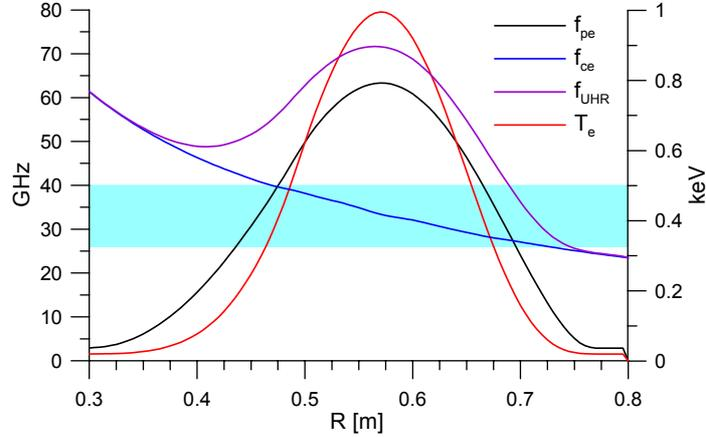
Fig. 2. Radial profiles of electron plasma frequency  $f_{pe}$ , electron cyclotron frequency  $f_{ce}$ , upper hybrid frequency  $f_{UHR}$ , and electron temperature  $T_e$ . COMPASS SND 1.2 T equilibrium computed by ACCOME.
