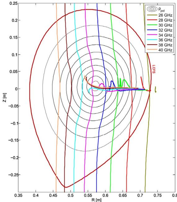
Fig. 3. Poloidal plasma cross-section of COMPASS with magnetic surfaces. Central ray trajectories for various frequencies and their respective electron cyclotron resonances are depicted.
