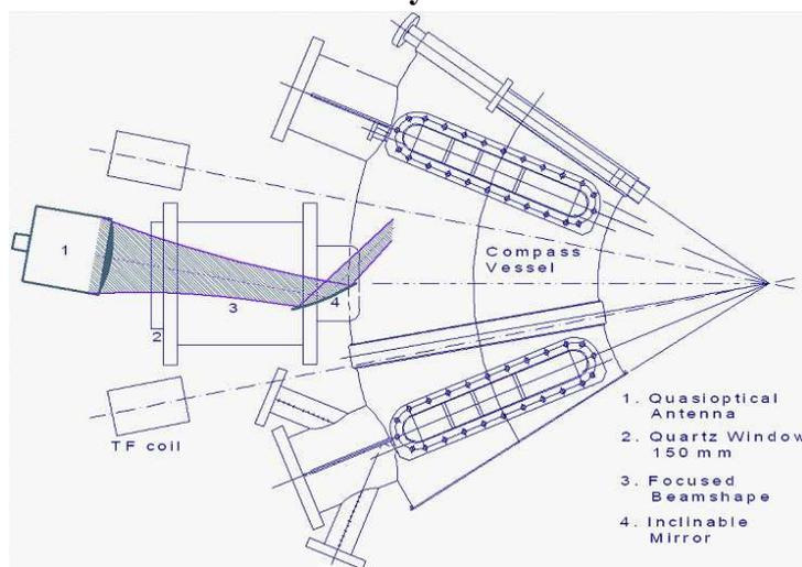
Fig 1 ECE antenna for 26-40GHz band
