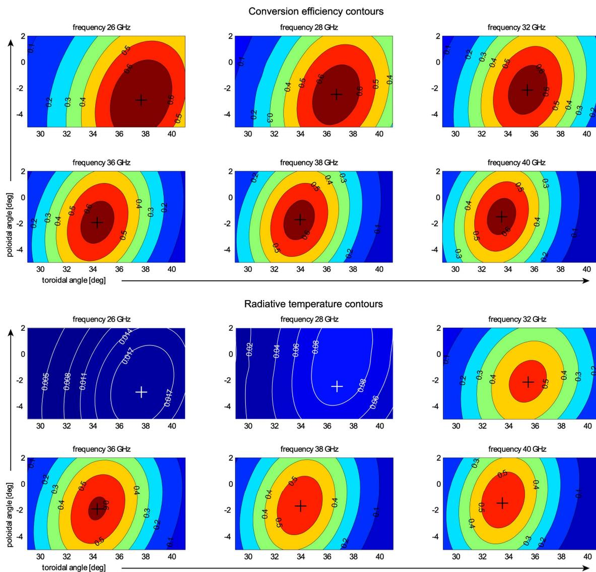
Fig. 5. Toroidal and poloidal angle scan of EBW-X-O conversion efficiency (top) and radiative temperature  $T_{\text{rad}}$  (bottom). Simulations were performed for the central rays only. Optimum angles for efficient conversion are marked by crosses.
