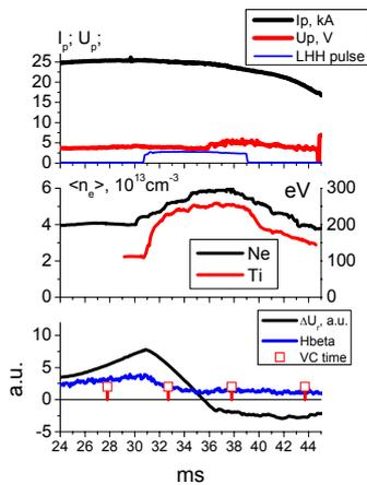
Fig. 5 The time history of the main experimental data. Moments of the video images are marked by red boxes.
