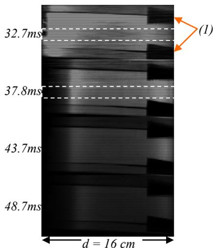
Fig.3 The sequence of the exposed plasma column images. Dashed lines selects the parts of the plasma column considered for profile intense graphics (see fig. 4).
