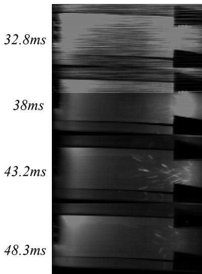
Fig. 6 Dust generation caused by micro breakdowns between the waveguides
