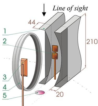
Fig.1 Interior of the chamber section with two waveguide LH grill
