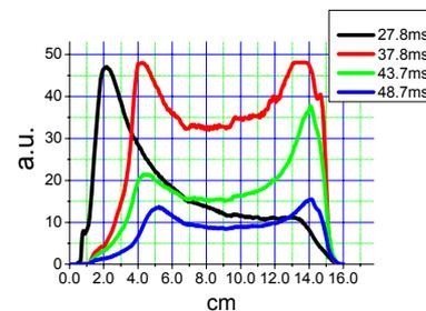
Fig. 4 Chord profiles of the plasma radiation for selected part (Fig. 3) of the plasma column.
