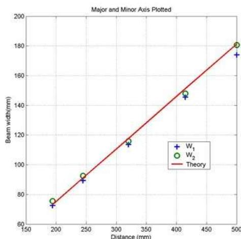
Fig. 1: Envelope of the beam leaving the horn. W1 and W2 should be identical, as the horn has a circular symmetry. The error is less than 3% between the measured beams in two orthogonal directions. The red line shows the expected divergence of the beam.
