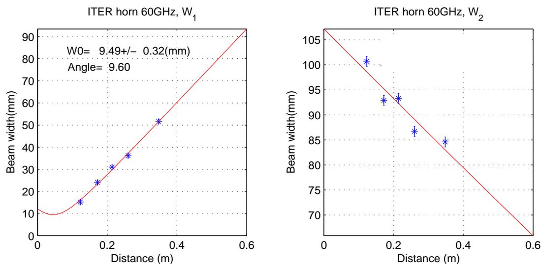
Fig. 3: Beam radius at various distances from mirror M1
