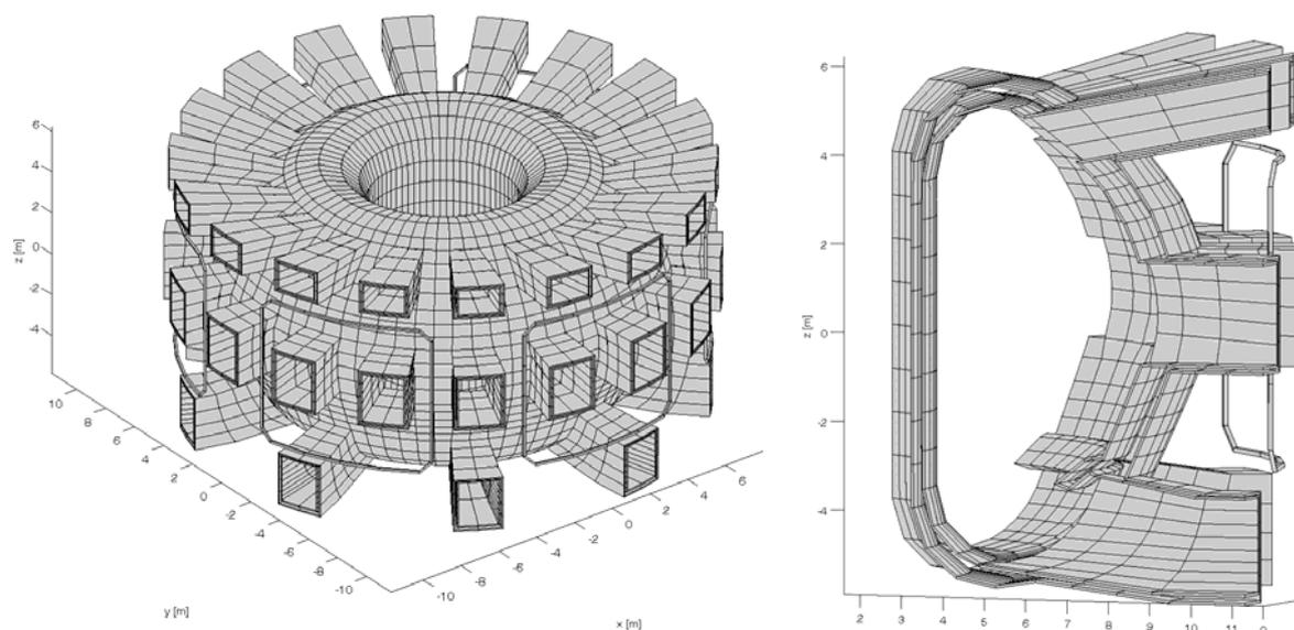
Fig. 1. Discretization of ITER geometry: overall view and cutaway figure.
