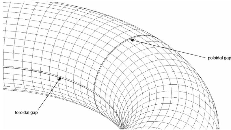
Fig. 2. Shell geometry and gaps as described in the mesh used in CarMa simulations.
