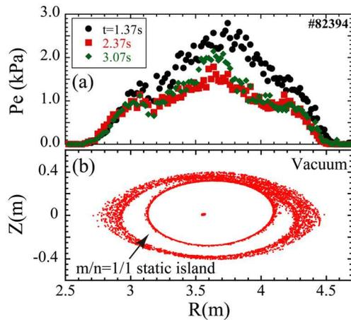
Fig. 3 (a) Electron pressure profiles of a discharge shown in Fig.2 obtained by Thomson scattering measurements. (b) Calculated Poincare plots of the vacuum field in the horizontally elongated cross section with  $I_{LID} / B_t = 1111 \text{ A/T}$ .
