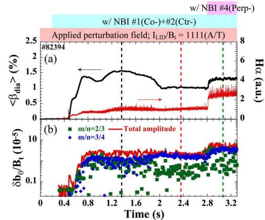
Fig. 2 Time evolution of an L-mode plasma with the applied large perturbation field. (a) Volume-averaged beta and H $\alpha$  signal. (b) Magnetic fluctuation amplitudes related to the edge MHD modes.
