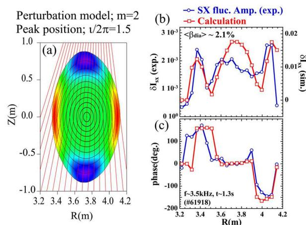
Fig. 1 Comparison of radial profile of SX fluctuation amplitudes of the  $m/n = 2/3$  mode between experimental observation and a simple perturbation model; (a) perturbation model and sight lines of an SX array, (b, c) experimentally obtained radial profiles of SX fluctuation amplitude and phase difference of the  $m/n = 2/3$  mode as a function of the SX sight lines.
