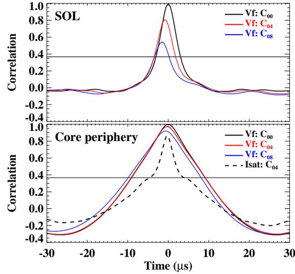
Figure 1: Floating potential cross-correlation for pins poloidally separated by 4 ( $C_{04}$ ) and 8 mm ( $C_{08}$ ) measured in the SOL and in the core periphery. The  $V_f$  auto-correlation is also shown ( $C_{00}$ ) as well as the  $I_{sat}$  cross-correlation in the core periphery.
