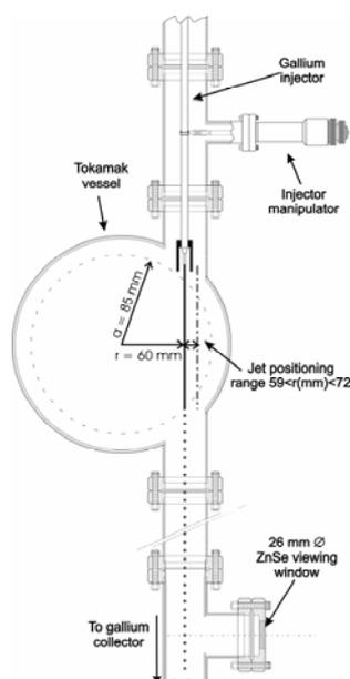
Figure 2: Schematic of the set-up in the vicinity of the plasma-jet interaction region
