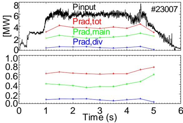
Fig. 2: Time evolution of the input power (black), total radiated power (red), radiated power in the main plasma (green) and in the divertor (blue) for the discharge from Fig. 1b. The upper picture shows absolute powers, the lower picture the fraction of the radiated power to the input power.
