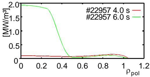
Fig. 5: Radiation profile in the main plasma as a function of the normalized flux radius during phases without ECRH heating (green) and with ECRH heating (red). The central radiation was kept successfully low by applying ECRH.
