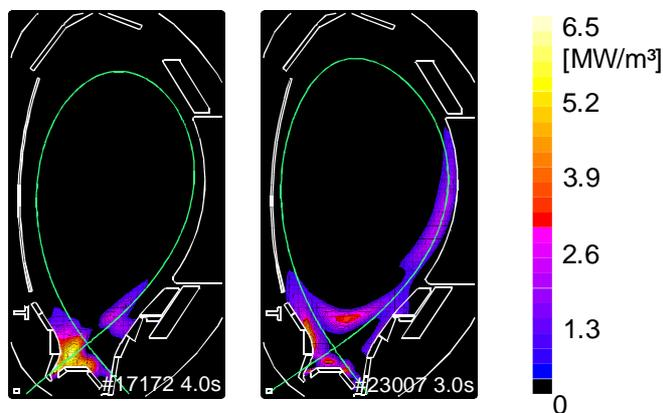
Fig. 1: Distribution of the radiation emissivity in a poloidal cross section of ASDEX Upgrade for two discharges with comparable plasma parameters. a) mostly carbon PFCs, b) full W covered PFCs
