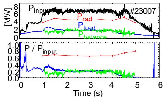
Fig. 4: Power balance for the discharge from figure 1b: Input power (black), total radiated power (red), power load to divertor tiles (blue) and power balance (green, see text) as absolute values (top) and as fractions to the input power (bottom)
