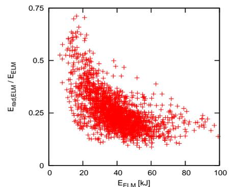
Fig. 6: Distribution of the normalized radiated energy due to a type-I ELM  $\Delta E_{\text{rad,ELM}}/E_{\text{ELM}}$  as a function of the ELM energy.
