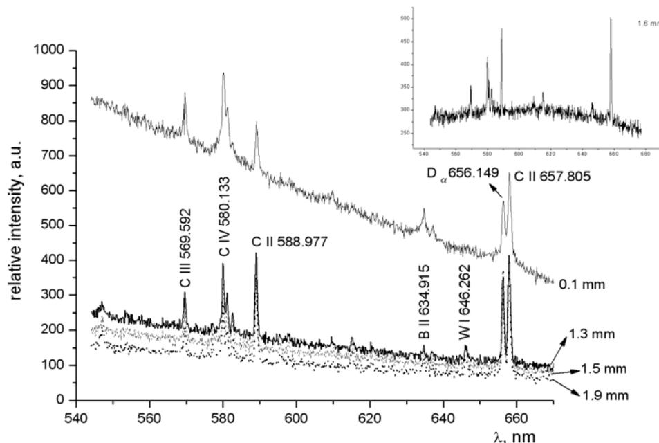
Fig.1. Spectra of laser-induced plasma at different distances from the ablation spark [8]
