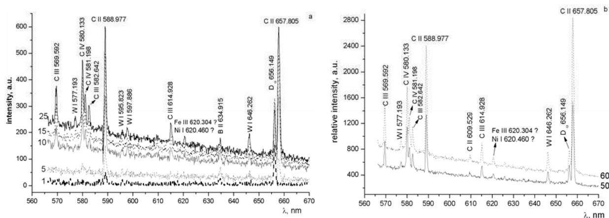
Fig.2a, b. Spectra after applying different numbers of laser pulses to the target. The numbers correspond to the number of the pulse in the sequence [6]
