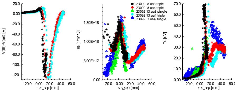
Figure 3: Divertor plasma parameters for ITER relevant conditions. Measurements of triple and single probes are shown.  $n_e$  and  $T_e$  measurements of triple probes are reliably for  $T_e \leq 30 eV$  only. The  $T_e$  peak of the triple probes at  $s - s_{sep} \approx 15 mm$  is an artefact.
