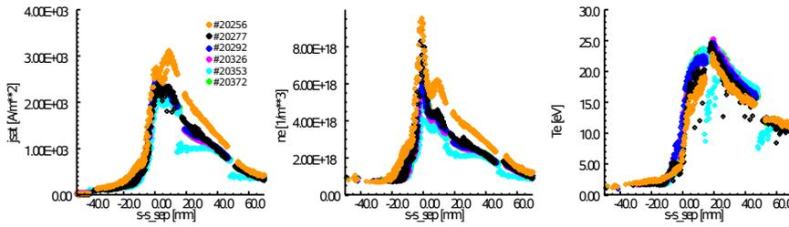
Figure 1: Influence of boronisation onto the divertor plasma at  $\bar{n}_e \approx 2.6 \times 10^{19} m^{-3}$
