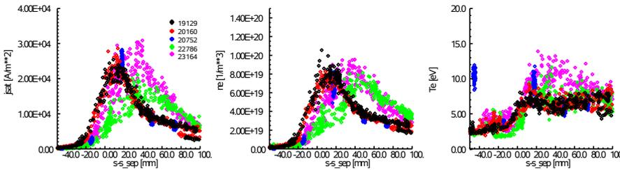
Figure 2: Divertor plasma parameter in H-mode for different levels of PFC W coating.
