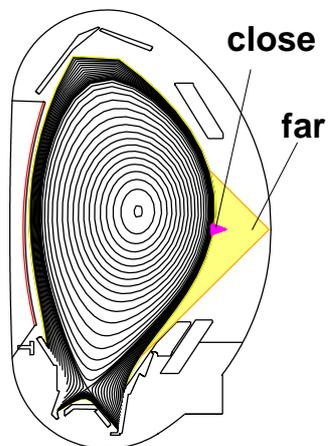
**Figure 1** (left). Target plasma and two valve configurations ("close" and "far").
