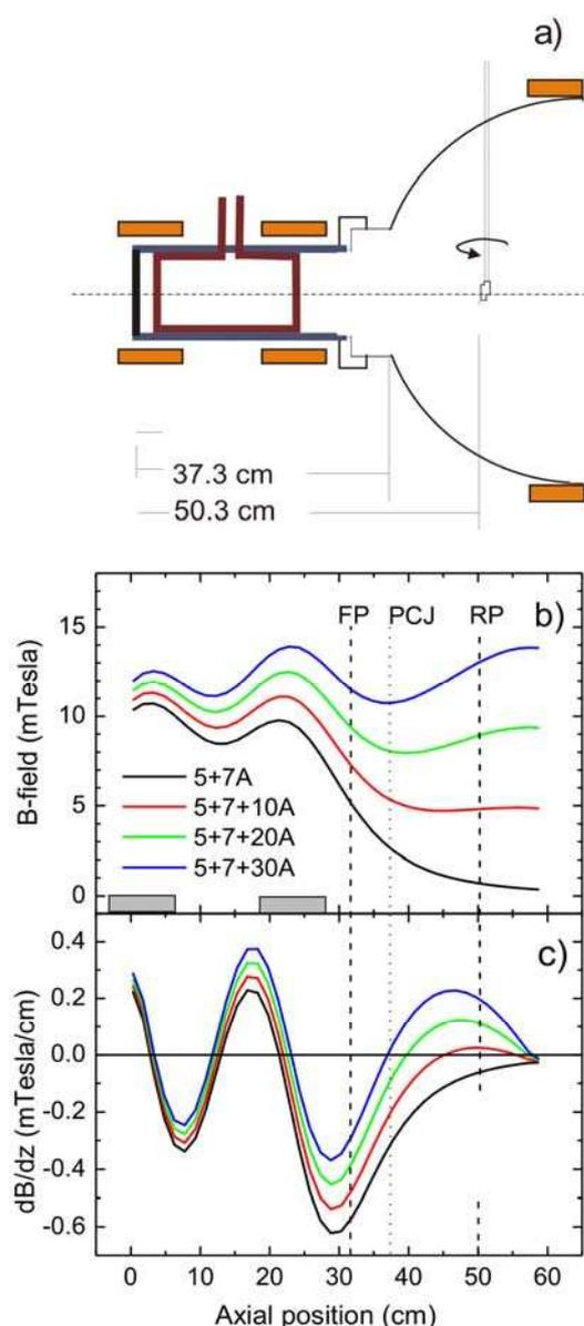
Figure 1. Sketch of the experimental setup a) with calculated magnetic field at the axis b) and its derivative c) for four different magnetic fields.
