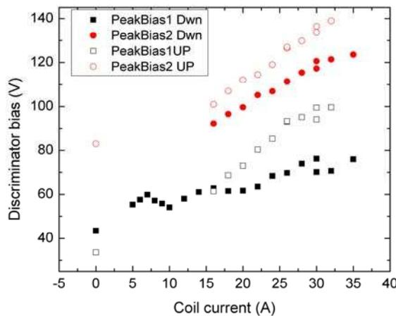
Figure 3. Discriminator bias for Gaussian peak fits of the IEDFs as a function of current in coil 3. Filled and open signal correspond to peaks in the IEDFs of the RFEA facing downstream and upstream directions, respectively. Black and red symbols represent low-energy and beam peaks, respectively.
