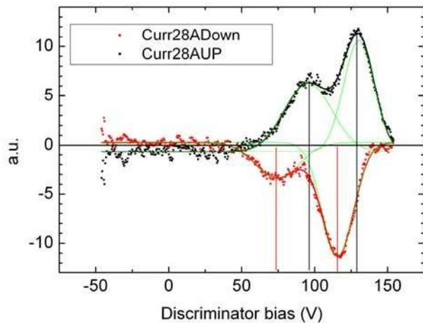
Figure 2. The IEDF of the RFEA facing the upstream plasma (black plot) and facing the downstream plasma (red, inverted plot). Dots corresponds to the derivative of the 7 points averaged RFEA current signal. Full lines represent the sum of the two fitted Gaussian peaks.
