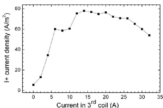
Figure 4. Ion saturation current vs. current in 3rd coil
