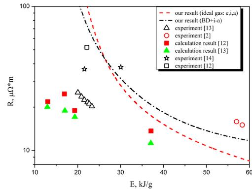
Figure 2: The electrical resistivity of aluminum vs the specific internal energy along isochore  $V/V_0 = 9$
