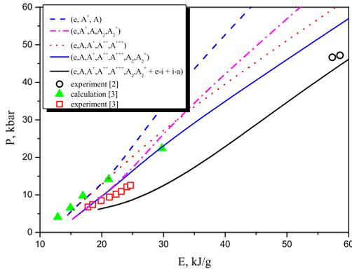
Figure 1: Pressure as a function of the specific internal energy along isochore  $V/V_0 = 9$
