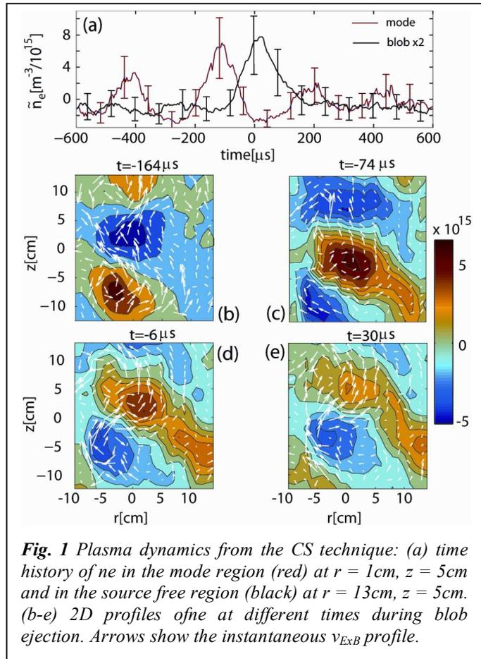
**Fig. 1** Plasma dynamics from the CS technique: (a) time history of  $n_e$  in the mode region (red) at  $r = 1 \text{ cm}$ ,  $z = 5 \text{ cm}$  and in the source free region (black) at  $r = 13 \text{ cm}$ ,  $z = 5 \text{ cm}$ . (b-e) 2D profiles of  $n_e$  at different times during blob ejection. Arrows show the instantaneous  $v_{\mathbf{ExB}}$  profile.
