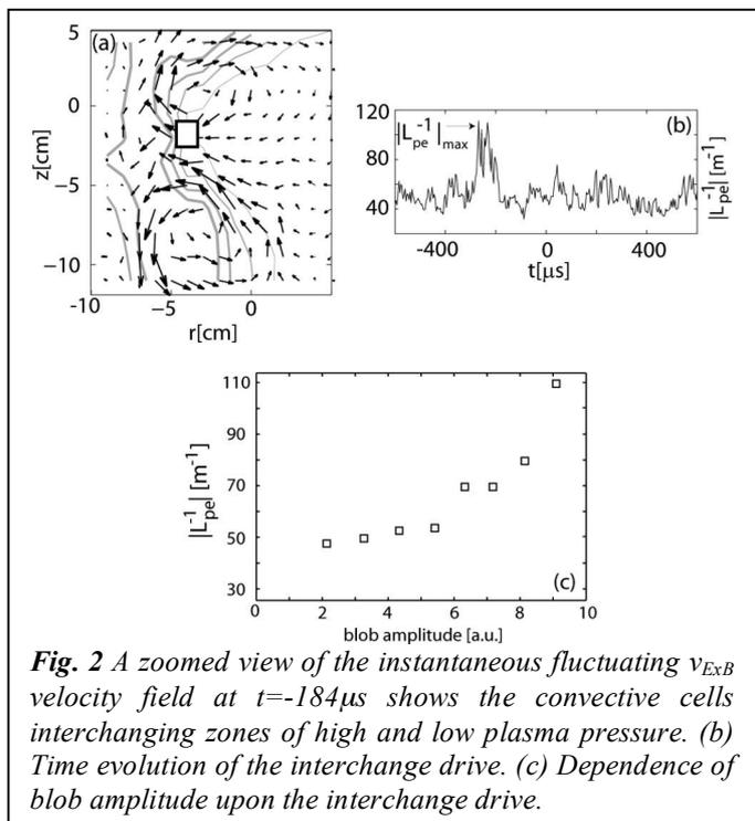
**Fig. 2** A zoomed view of the instantaneous fluctuating  $v_{\mathbf{ExB}}$  velocity field at  $t = -184 \mu\text{s}$  shows the convective cells interchanging zones of high and low plasma pressure. (b) Time evolution of the interchange drive. (c) Dependence of blob amplitude upon the interchange drive.
