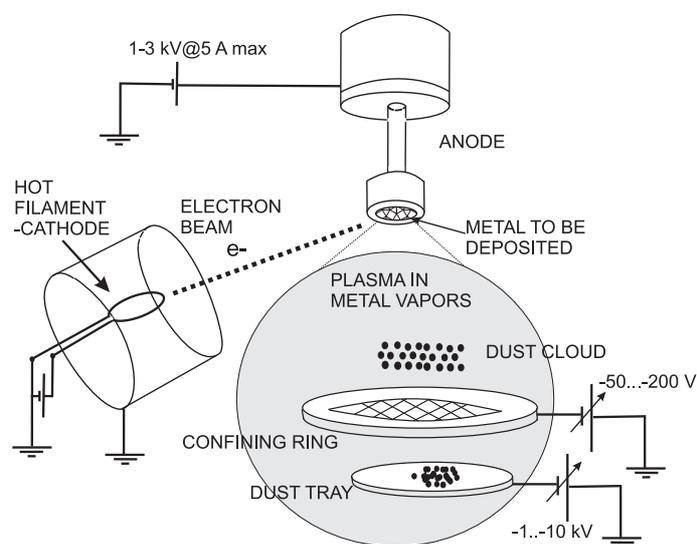
Figure 1: Proposed set-up for dust coating in vacuum arc plasma
