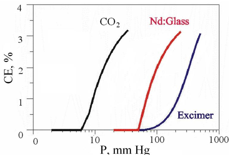
**Fig.3.** Conditions of generation of EUV radiation for three lasers. Dependence of conversion efficiency on Xe gas target pressure.
