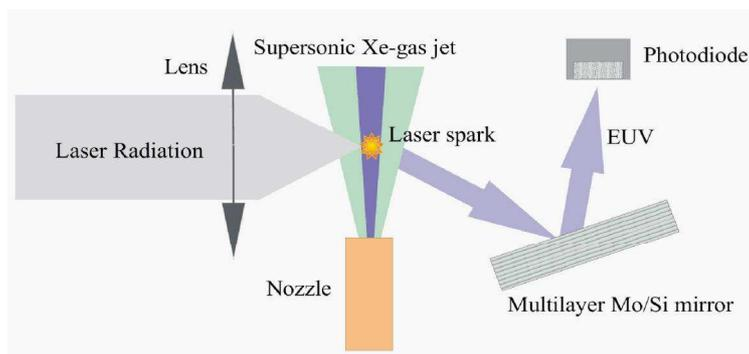
Fig.1. Scheme of gas-jet EUV source.
