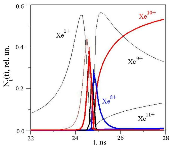
Fig.2. Ionization dynamics of LPP in xenon.
