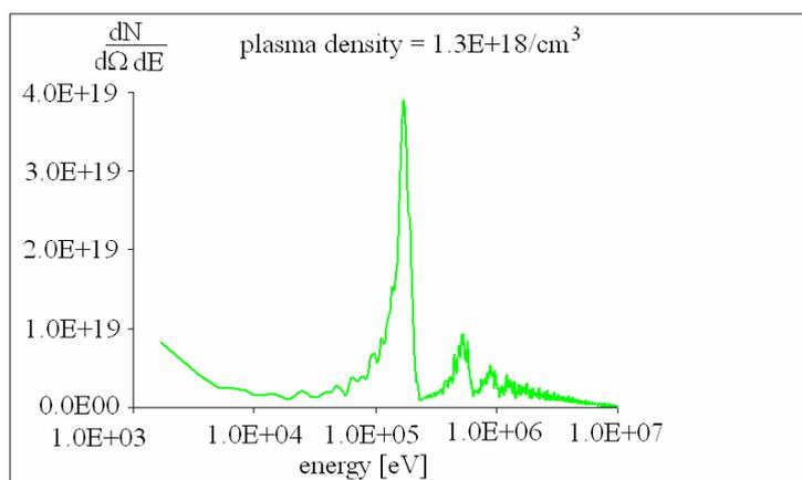
Figure 3: Betatron radiation energy spectrum on-axis. The differential number of photons emitted is plotted as a function of the energy.
