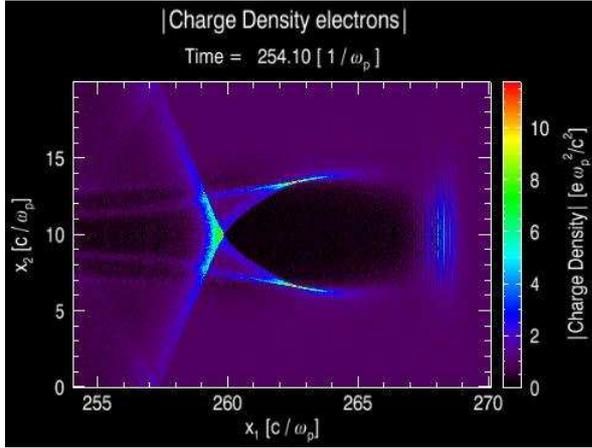
Figure 1: On-axis cut of the electron density in bubble regime conditions. The simulations have been performed using the OSIRIS code [4]
