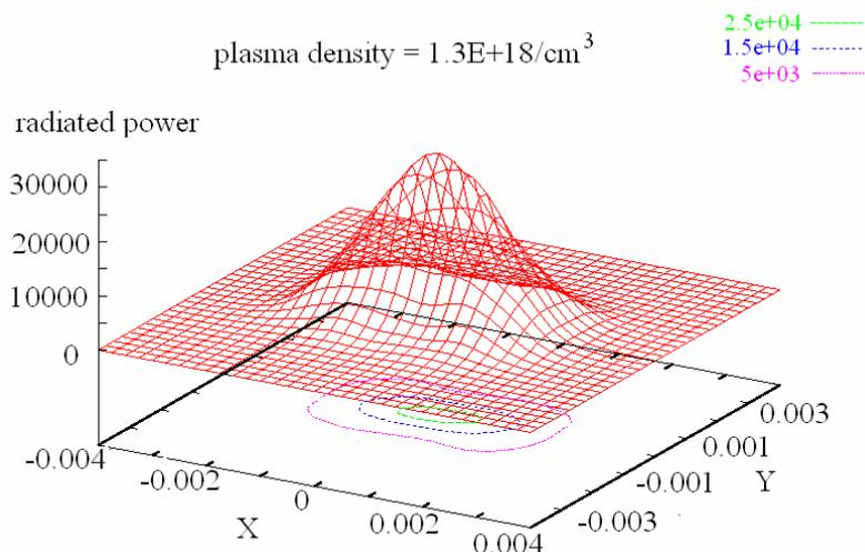
Figure 3: Spatial distribution of betatron radiation calculated for plasma density= $1.3 \cdot 10^{18} \text{ cm}^3$ .
