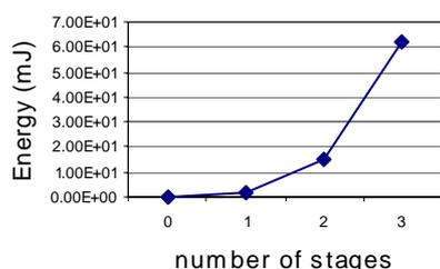
Figure 3. Energy amplification with three stages. The seeded energy was  $1.0e-4$  mJ
