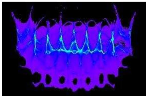
Figure 2 X-ray laser output amplified by an inhomogeneous plasma created in a rugous target
