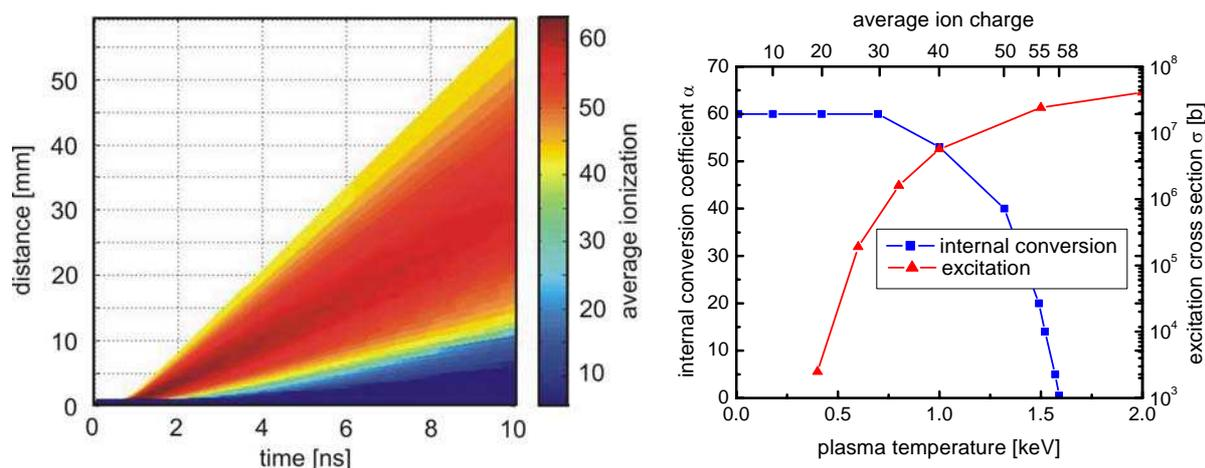
Fig. 2. Temporal and spatial distributions of Ta plasma ionization (left) influence considerably the  $^{181}\text{Ta}$  nuclear level excitation and number of activated nuclei decaying via emission of 6.2-keV photons (right).
