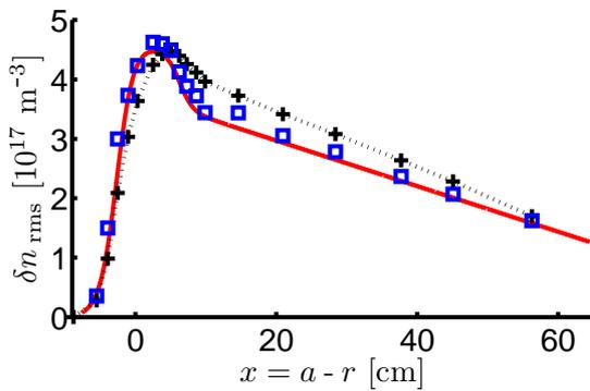
Figure 4: Black crosses: fluctuation level deduced from the  $\sigma^2$  data of Fig. 3 using Eqs. (1) and (3). The linear interpolation is overplotted using a dotted line, and  $\delta n_{\text{rms}} = 0$  was introduced artificially at the edge on the left. Blue square symbols: Result of the optimisation algorithm that uses Eq. (2). The input profile is displayed with solid red line for comparison.
