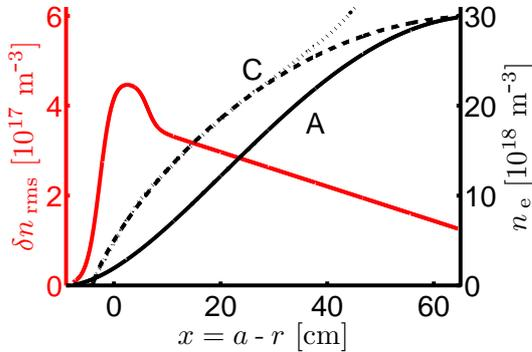
Figure 2: Input profiles for the Full-Wave simulation. Red: model for the fluctuation level  $\delta n_{\text{rms}} = \sqrt{\langle \delta n^2 \rangle}$  based on data from Tore Supra # 38316. Black: density profile models A (concave) and C (convex). Dotted line: profile measured in Tore Supra # 38316.  $r$ : radial profile coordinate.  $a$ : radius of the plasma boundary.
