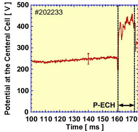
FIG. 2. Temporal evolution of the potential measured by GNPB. This data was obtained at the fixed position of  $r = 0$  cm.
