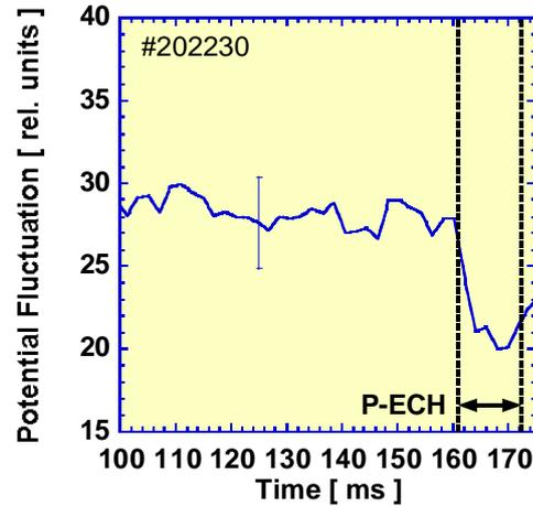
FIG. 3. Temporal evolution of FFT fluctuation of potential.
