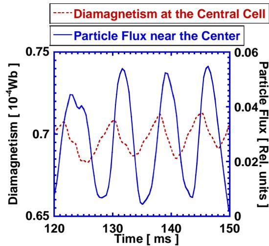
FIG. 5. Temporal evolution of diamagnetism and radial flux due to the phase difference between potential and density fluctuations.
