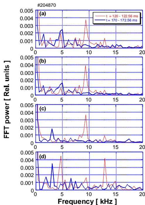
FIG. 1. FFT spectra of each channel before ECH (hair line,  $t = 120\text{--}122.56$  ms) and during ECH (solid line,  $t = 170\text{--}172.56$  ms) are shown in FIG. 1 (a) at horizontal position of 0 m, (b) at 0.03 m, (c) at 0.06 m, and (d) at 0.09 m, respectively.
