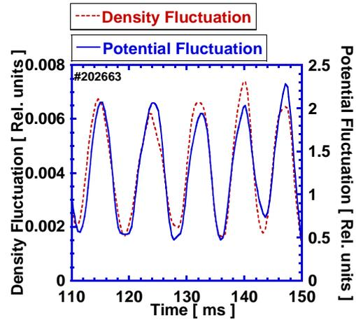
FIG. 4. Temporal evolution of the low-frequency potential oscillation and the density oscillation near the central of GAMMA
