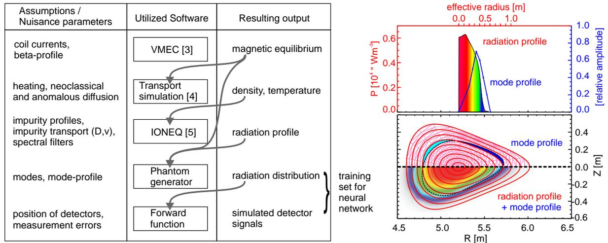
**Figure 1:** Left: Simulation software chain used to create the inputs and outputs for training the NNs. Dependencies and nuisance parameters are also listed. Right:  $m=2$  mode perturbs the magnetic flux-surfaces (VMEC output). The radiation profile (from IONEQ) is mapped onto these perturbed flux-surfaces.
