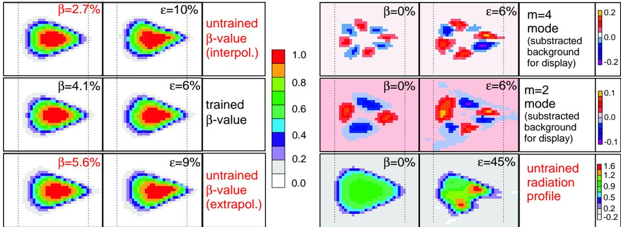
Figure 2: Left: comparison between phantom and reconstruction data for selected phantoms with different  $\beta$ -values. Right: comparison of mode reconstruction and a failing reconstruction for a phantom with a different (untrained) radiation profile.
