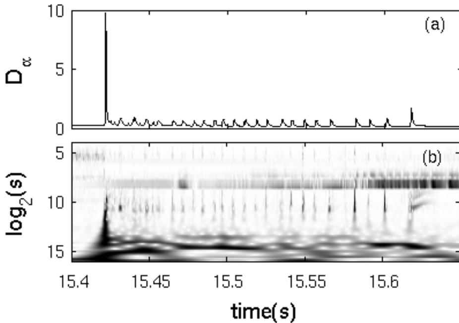
**Figure 1.** JET pulse #58982:(a)  $D_\alpha$  emission signal; (b) Normalised wavelet coefficients, computed from the Mirnov coil data. Frequency is related to the scale  $s$  via  $\omega = 2\pi/(s \cdot \delta t)$ .
