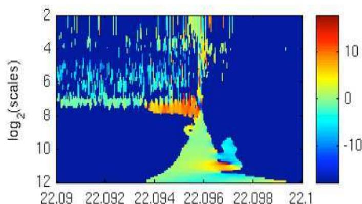
**Figure 4.** Morlet spectrogram of magnetic perturbations showing the toroidal mode numbers of an ELM precursor and ELM in JET pulse #53062 [5].
