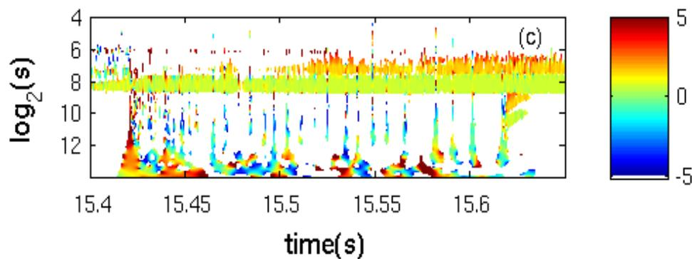
**Figure 2.** Toroidal mode number  $n$ , extracted from the phase shift between magnetic perturbation measured with two edge Mirnov coils with toroidal separation of 10.17 degrees. The color scale is saturated between  $[-5,5]$ , modes with  $n > 5$  are shown as deep red.
