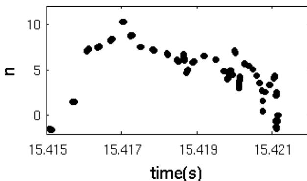
**Figure 3.** Time evolution of the toroidal mode number for a constant level of power spectral amplitude extracted from of two Mirnov coils toroidally separated by 10.17 degrees.
