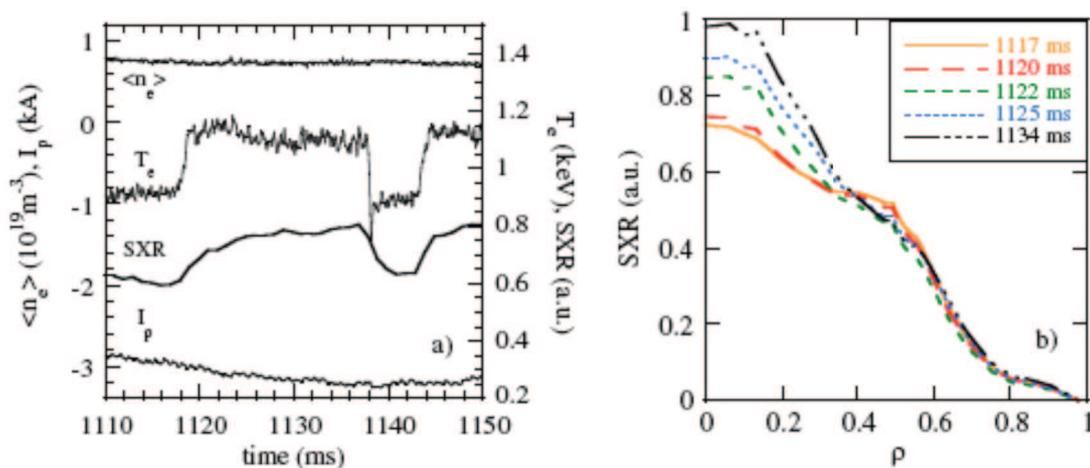
**Figure 2.** Time evolution of plasma current, line density, central temperature and SXR signal (left). Time evolution of electron temperature profile as measured by ECE (right).
