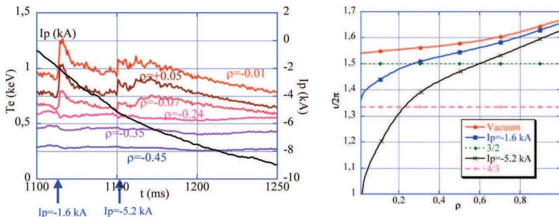
**Figure 1.** Temperature given by ECE measurements (left) and rotational transform profile (right) evolution during an OH-induced current experiment in TJ-II. The rotational transform profiles are shown for the times when the CERC is triggered.
