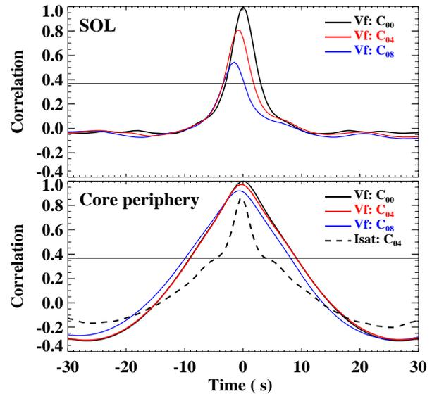
*Figure 1: Floating potential cross-correlation for pins poloidally separated by 4 ( $C_{04}$ ) and 8 mm ( $C_{08}$ ) in the SOL and in the core periphery. The  $V_f$  auto-correlation is also shown ( $C_{00}$ ) as well as the  $I_{sat}$  cross-correlation in the core periphery.*
