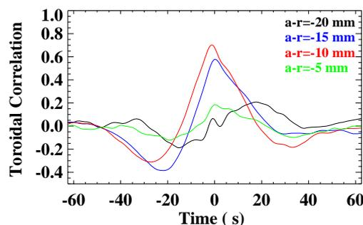
*Figure 3: Cross-correlation function for floating potential signals measured between the poloidal probe located at  $r-a = -10$  mm and some of the pins of the rake probe.*
