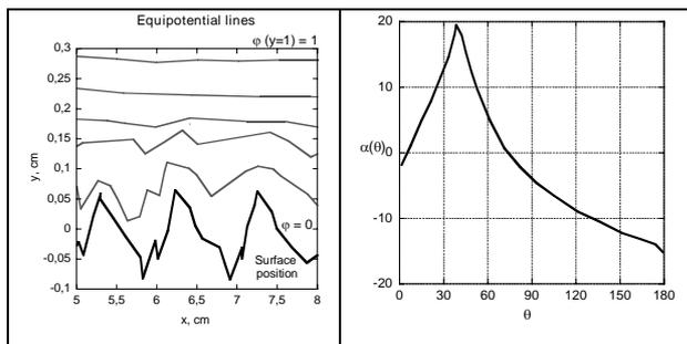
Fig. 3 Calculated equipotential lines over the rough surface.
