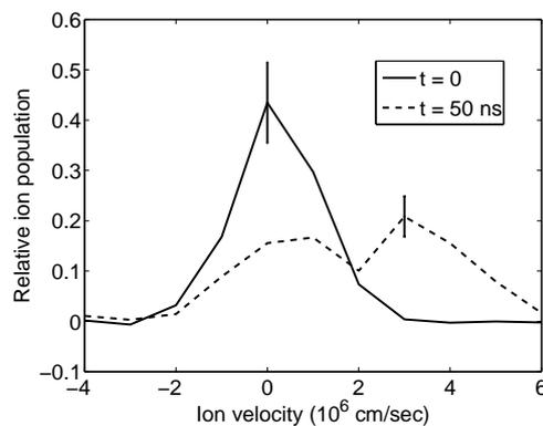
Figure 2: Ion velocity distribution before and after the magnetic field penetration.
