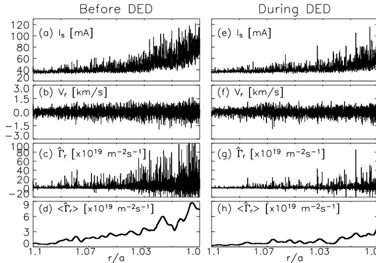
Fig. 4 Comparison of the  $I_s$ ,  $V_r$  and  $\tilde{T}_r$  signals (versus normalized radial position) measured in the SOL before (left column) and during (right column) the static 6/2 DED (# 101795). Plotted in (d) and (h) are the ensemble-averaged turbulent flux. Corresponding parameters in the two columns are drawn in the same scale.
