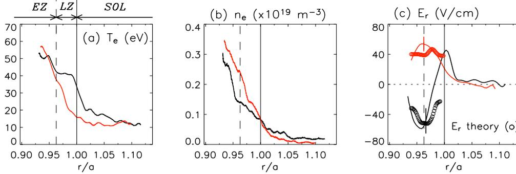
Fig. 1 Radial profiles of (a) electron temperature; (b) plasma density and (c) radial electric field before (black solid curves, w/o RMP) and during (red solid curves, with RMP) the static 6/2 DED measured by fast reciprocating probes at TEXTOR (# 99626). The radial locations are normalized by  $a$ . The vertical dashed line roughly separates the ergodic zone (EZ, left side) and the laminar zone (LZ, right side). The open circles in (c) show the simulated  $E_r$ .
