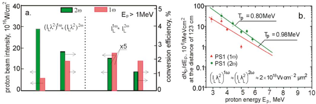
Fig. 2. A comparison of parameters of moderate-energy (1 – 3MeV) (a) and high-energy ( $>3\text{MeV}$ ) (b) proton beams generated by a  $1\omega$  or  $2\omega$  laser beam.  $I_L^{1\omega} \approx 2 \times 10^{18} \text{W/cm}^2$ . For part (b): points – the results of SSTD measurements, lines – the results of approximation by the Maxwellian energy distribution with the temperature  $T_p$ .
