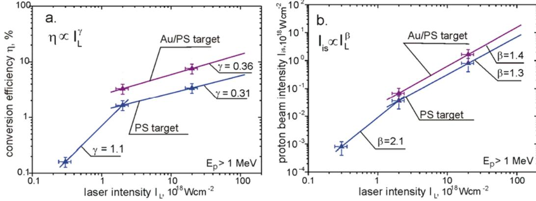
Fig. 1. The laser-protons energy conversion efficiency and the proton beam intensity at the source as a function of laser intensity for PS and Au/PS targets. Points – the results of IC measurements, lines – the results of approximation by a power function.
