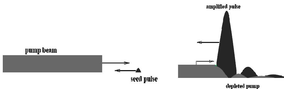
fig.:1 Principle of amplification of counterpropagating beams
