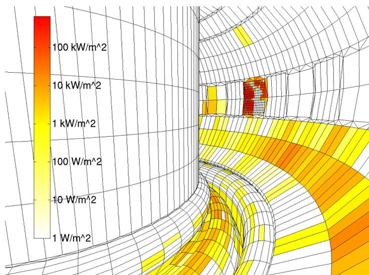
Figure 1: Power load to the wall tiles due to alpha particles produced in thermonuclear reactions in ITER *Sce-2* plasma with uncompensated ripple.
