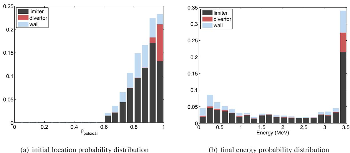
Figure 2: The distributions of a) the initial location and b) the final energy. The probabilities of a limiter hit, a divertor hit and a regular wall hit are separated by color.
