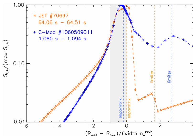
Fig.4 Normalised ionisation source rates from KN1D for pedestal-top identity shot pair. The abscissa is centred on the density pedestal foot in each case and normalised by its width, ie the shaded region denotes the main gradient zone. Separatrices and boundary surfaces (“limiter”) of respective KN1D grids indicated by dashed lines.
