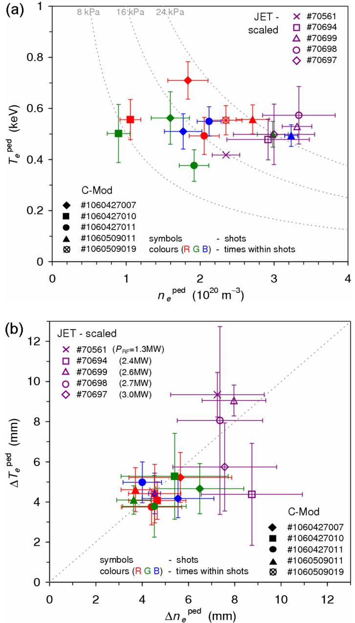
Fig.3 (a) Pedestal heights interpolated for C-Mod / JET power scans, JET data scaled onto C-Mod ranges (cf Table 1). Best matches implying edge dimensionless identity obtained for higher densities. (b) Accompanying pedestal widths, JET data scaled with size ratio.
