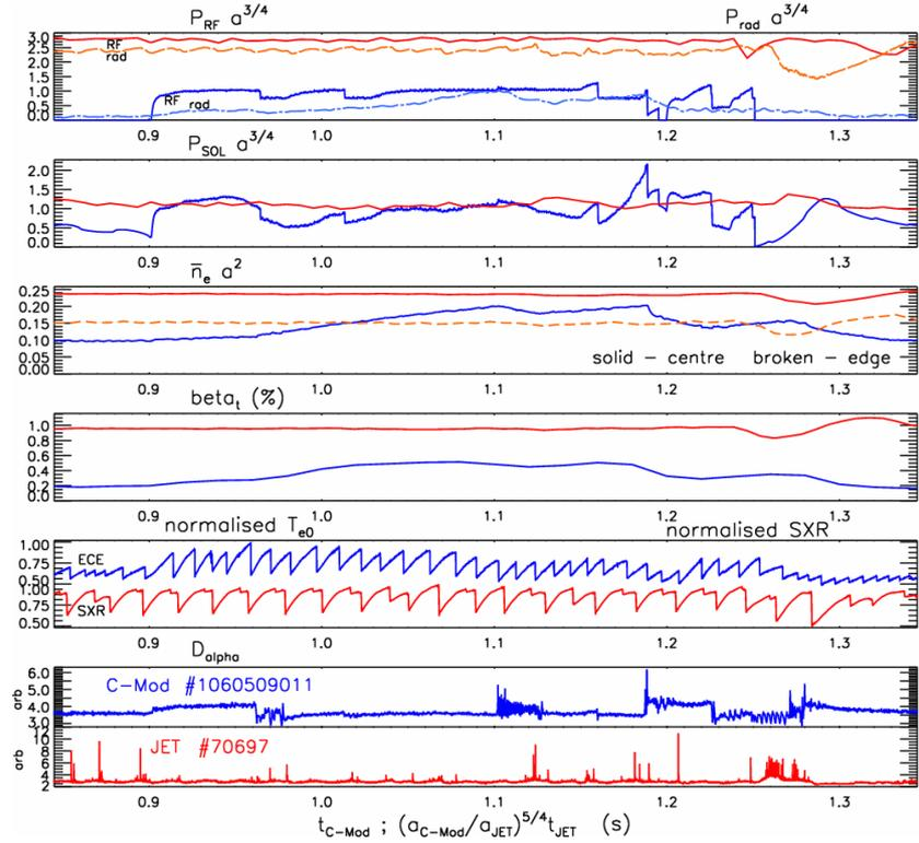
Fig.2 Global quantities (scaled powers and densities,  $\beta_t$ , sawtooth oscillations,  $D\alpha$  emission) for C-Mod / JET shot pair with close dimensionless identity at the pedestal top. JET signals scaled onto time axis of C-Mod (see text).
