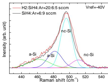
Fig. 1 Raman spectra of the nc-Si films by HNB CVD and.
