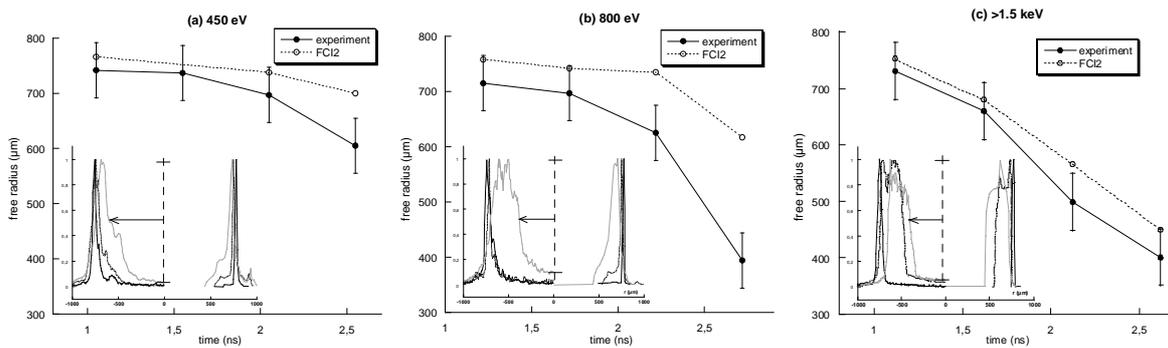
**Figure 3** : Time resolved measurements of free radius for a gas-filled hohlraum in all three spectral ranges. Insets at the left bottom of each plot show experimental (left) and simulated (right) profiles at 1ns, 2ns and 2.5ns. Arrows oriented to the left in the insets illustrate the definition of the free radius at 2.5ns.
