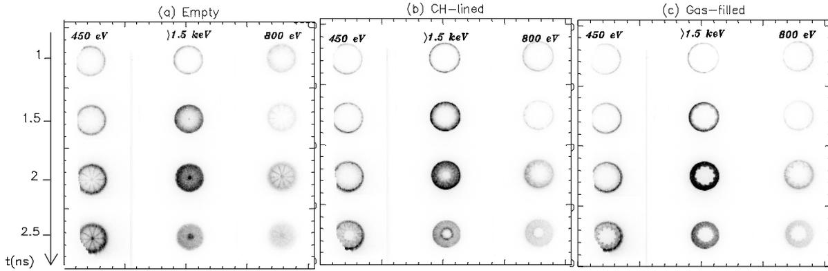
**Figure 2** : On-axis imagery of (a) empty, (b) CH-lined and (c) gas-filled hohlraums.
