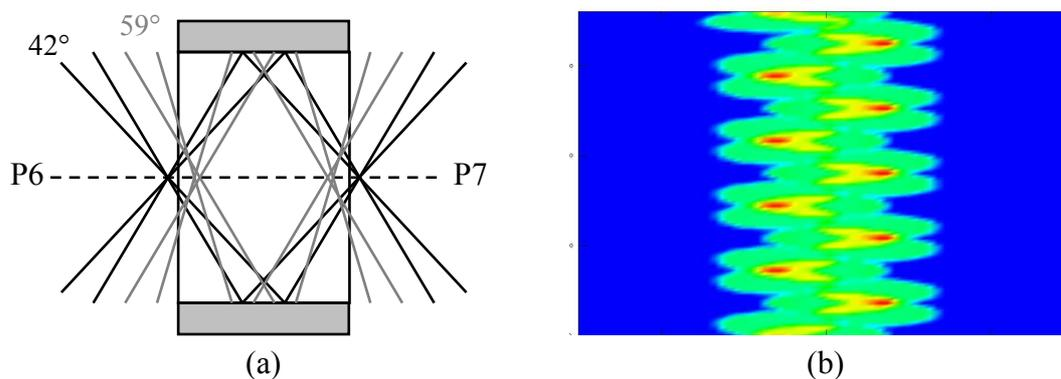
*Figure 1 : (a) irradiation geometry scheme, (b) resulting initial hotspots in the  $z$ - $\theta$  plane calculated with VISRAD.*
