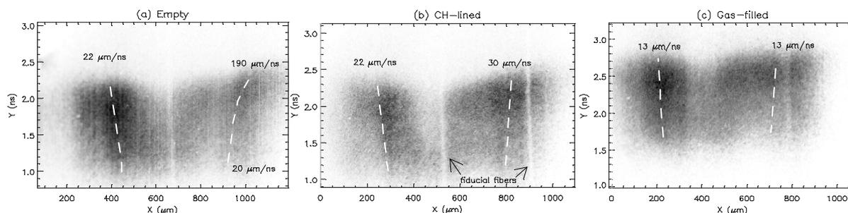
*Figure 4 : Streaked perpendicular imaging of laser spots as seen through the thinned wall of the different kinds of hohlraums that were shot. White dashes illustrate trajectories of hot spots with their average speeds.*
