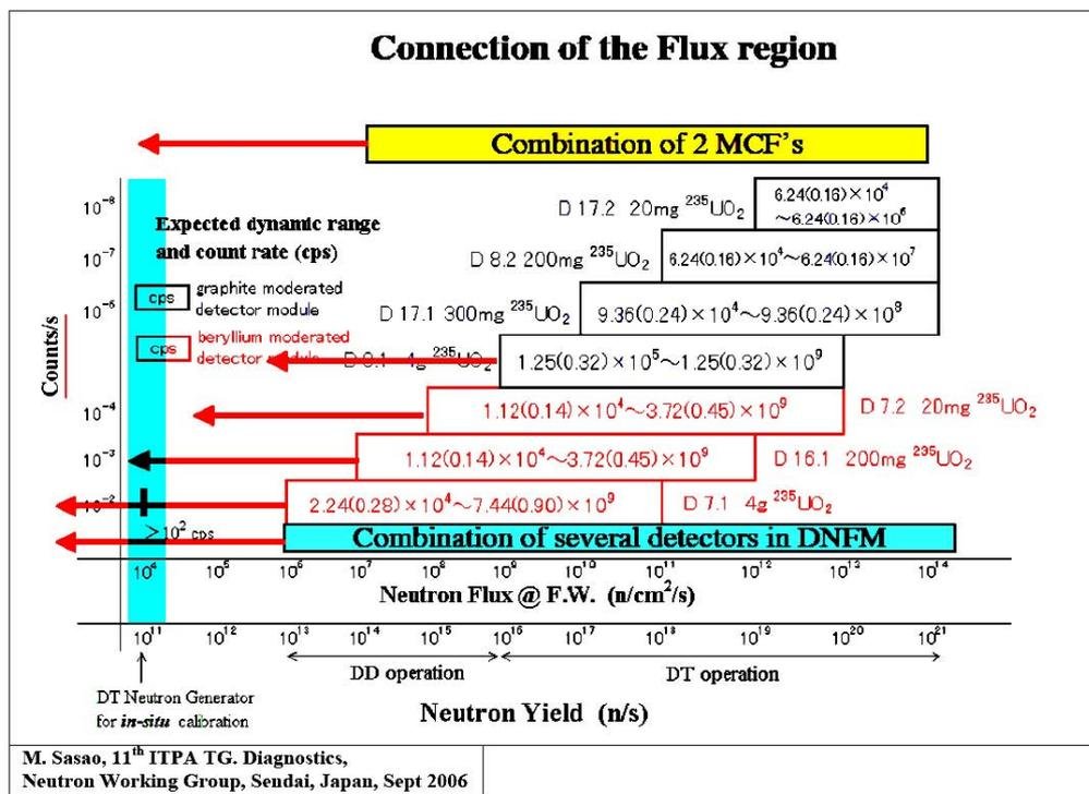
Fig. 1. ITER neutron emission range and how it will be covered by the different proposed detectors.
