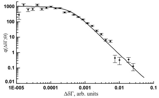
**Figure 2.** PDF of increments of amplitudes  $\tilde{\Gamma}^*$  in the ECR heated plasma. Points show the empirical distribution, a solid curves shows the FSD with parameters  $\Theta = (\alpha, \beta, \theta, \lambda)$ , where  $\alpha = 1.11$ ,  $\beta = 0.96$ ,  $\theta = 0$ ,  $\lambda = 0.00033$ .
