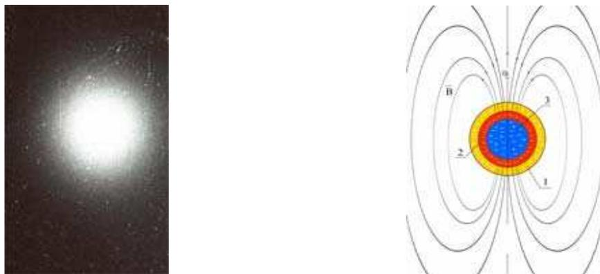
Fig.1 On the left - laboratory ball lightning image 25 cm in diameter at the distance of 2,5 m upwards from a discharge cell. Exposure – 20 ns. Storage capacity – 200 microfarad. On the right - ball lightning structure. Symbols: 1 – external ringular layer; 2 – intermediate layer; 3 – kernel;  $\vec{B}$  – lines induction of magnetic field.
