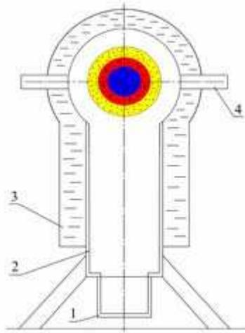
Fig.2. The scheme of reactor on base of ball lightning. Designations: 1-discharge cell; 2-chamber; 3- blanket; 4- devices for heating.
