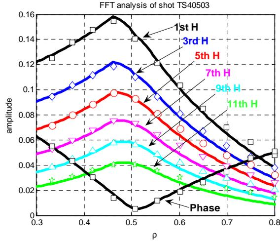
Fig.2 Amplitudes of harmonics 1, 3, 5, 7, 9, 11 of the Fourier transform of the modulated temperature. The points represent the experimental values, the solid lines represent the simulation.
