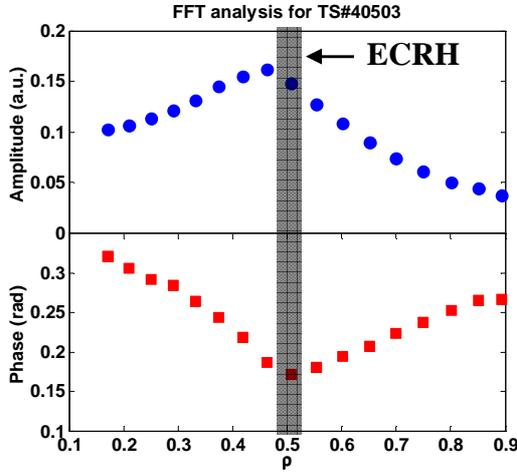
Fig.1 Phase and amplitude of the 1<sup>st</sup> harmonic of the Fourier transform of the modulated temperature.
