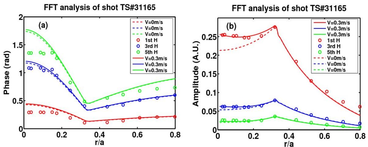
Fig.5 Phase (a) and amplitude (b) of the 1<sup>st</sup>, 3<sup>rd</sup>, 5<sup>th</sup> harmonics of the Fourier transform of the modulated temperature. Simulations with pinch (solid) and without pinch (dash).
