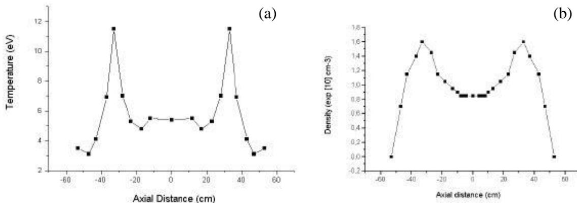
Fig 02 Axial electron plasma temperature(a) and density (b) space profile.
