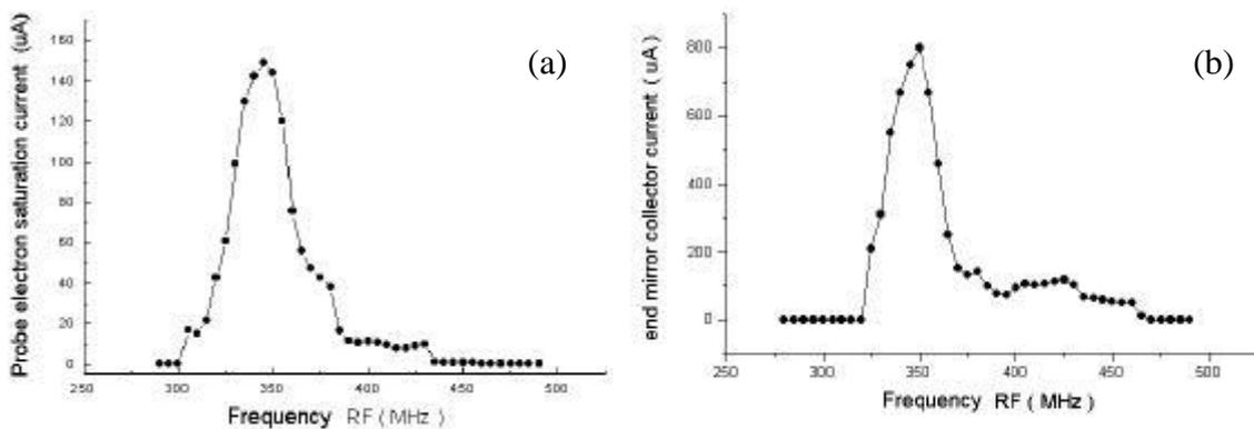
Fig. 03. (a) Electron saturation current versus RF frequency detected by aLangmuir probe.
