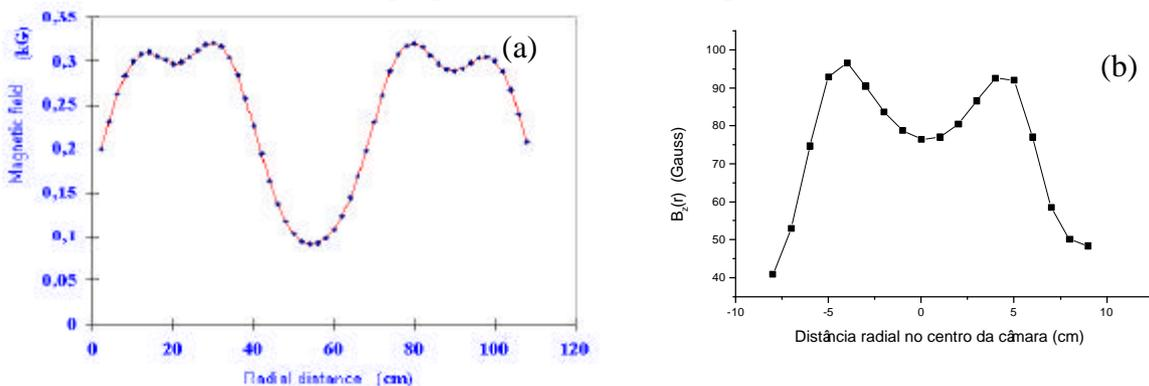
Fig. 01 (a) Axial space profile of the magnetic field (b) Radial space profile of the magnetic field. ( Measured by Hall probes)
