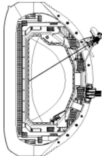
Fig. 1. The present DISRAD diagnostic has a single viewing chord through the DIII-D plasma.
