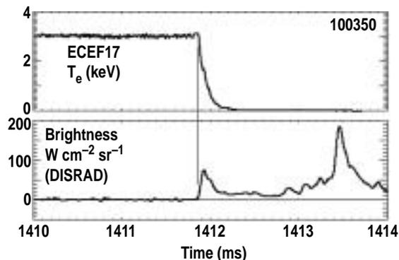
Fig. 4. In the thermal quench, decay time of  $T_e$  and radiant power are similar.
