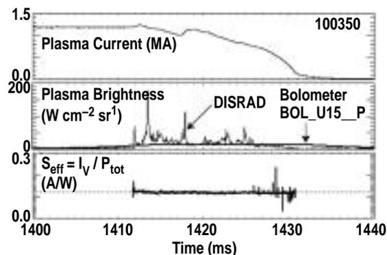
Fig. 3. The DISRAD diagnostic provides good temporal resolution of radiant power during disruptions. The time integral (radiated energy) agrees with the bolometer.
