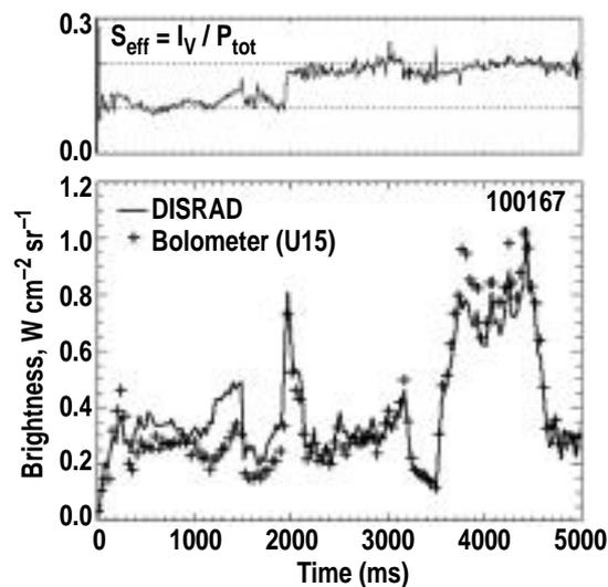
Fig. 5. Agreement with bolometer is found also in quasi-steady plasmas. The effective responsivity is less constant than in disruptions.
