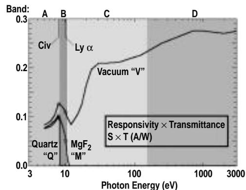
Fig. 2. The AXUV photodiode responsivity (V curve) varies significantly below 22 eV photon energy. The M and Q curves include the filter transmittance. Four spectral regions (A, B, C, D) are identified for analysis.
