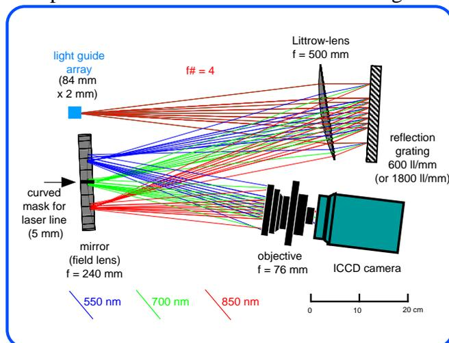
Fig. 2: Setup of Littrow-type spectrometer
