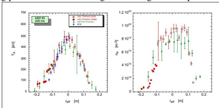
Fig. 4: Electron temperature and density profiles measured by ruby Thomson scattering (red squares), Nd:YAG Thomson scattering (green triangles) and ECE diagnostic (blue circles).
