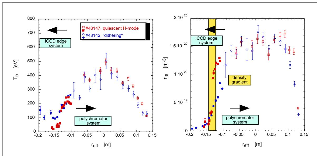
Fig. 5: Electron temperature and density profiles in a dithering (blue circles) and a quiescent H mode phase (red squares). Measured by ruby Thomson scattering diagnostic (full symbols denote data from the new CCD diagnostic).
