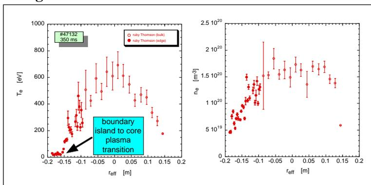
Fig. 6: Electron temperature and density profiles in a discharge with high edge density
