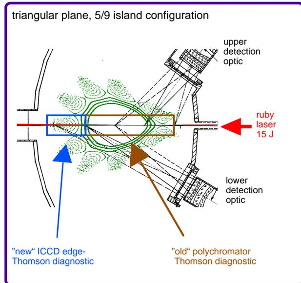
Fig. 1: Partitioning of the view chord. The total length of the view chord is 420 mm.
