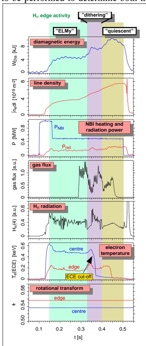
Fig. 3: Overview of discharge parameters for the investigated H-mode discharges.
