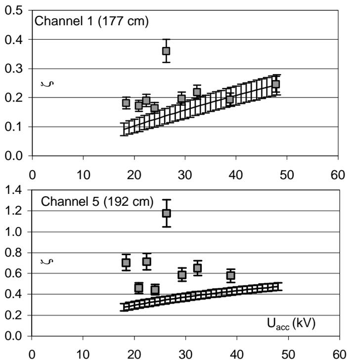
Figure 3: Beam attenuation of the full energy component in three locations. The attenuation code results are represented by the line with error bars, the BES measurements by the squares with error bars.
