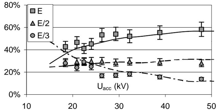
Figure 2: Injected power fractions. Comparison of the BES measurements of the outermost channel (error bars) and the testbed results (lines). We can see a good agreement.
