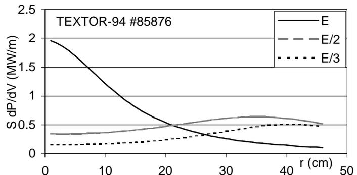
Figure 5: Power deposition profiles measured with BES. The components E, E/2 and E/3 are presented. We have taken the Shafranov shift into account.
