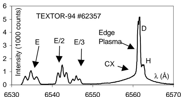
Figure 1:  $H_{\alpha}$  spectrum emitted by a tokamak plasma. We can clearly separate the passive part, consisting of the Charge Exchange pedestal and the Plasma Edge emission, from the active part, emitted by the neutral beam atoms. Both the Zeeman splitting of the edge spectrum and the Motional Stark Effect of the beam spectrum are visible.
