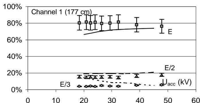
Figure 4: Relative abundance for the power fractions for a central channel. The figure shows testbed and beam attenuation code predictions (lines), BES measurements (black markers) and fit results (white markers with error bars). We notice a fair agreement between the predictions and the fit results.
